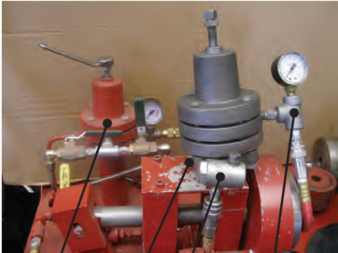
CONTROL REGULATOR OUTPUT SUPPLY CONTROLLED PRESSURE
